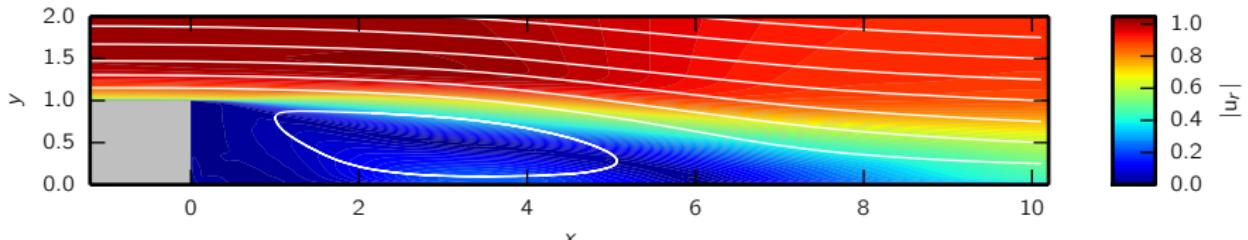
Streamwise velocity error RANS-SA (top) vs. RANS-SA- $\beta(x)$  (bottom)
